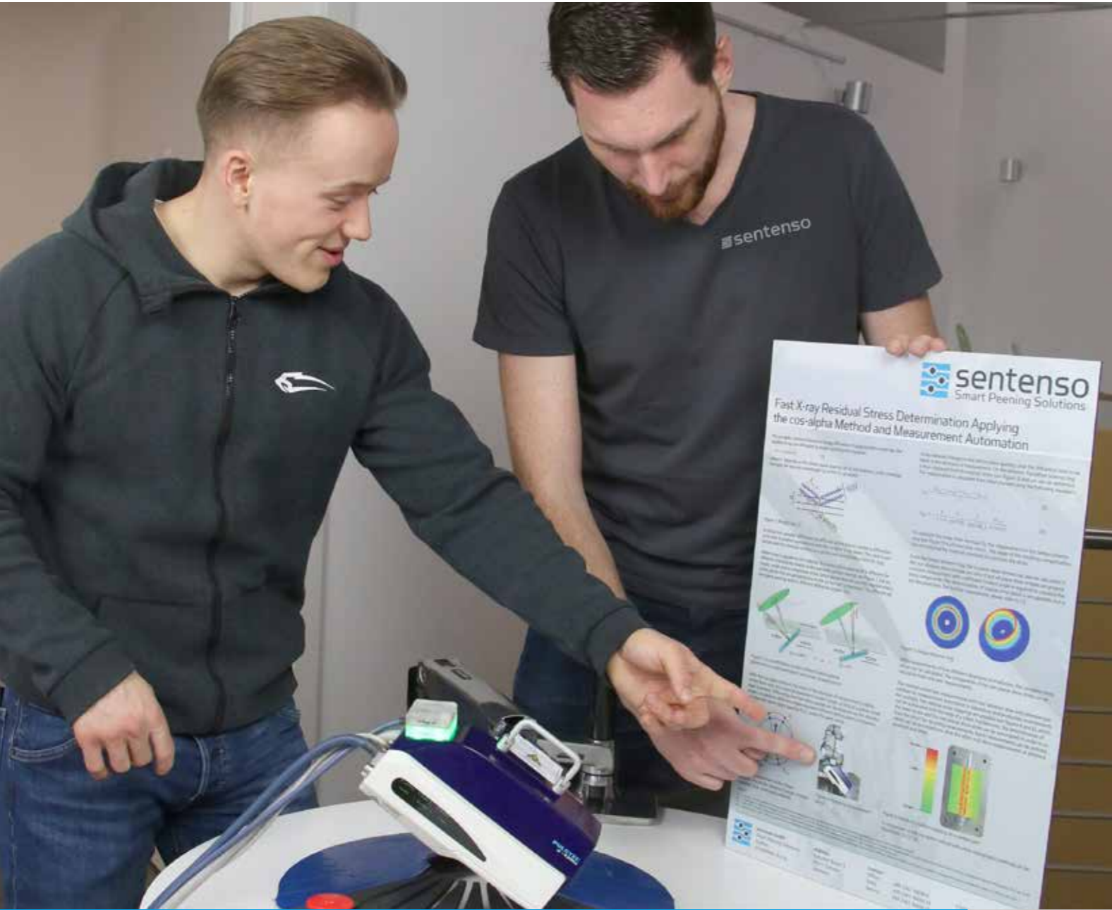
New Ways and Fast Results in X-ray Diffraction Basic understanding and practical determination of residual stresses with the X-ray stress analyser.
