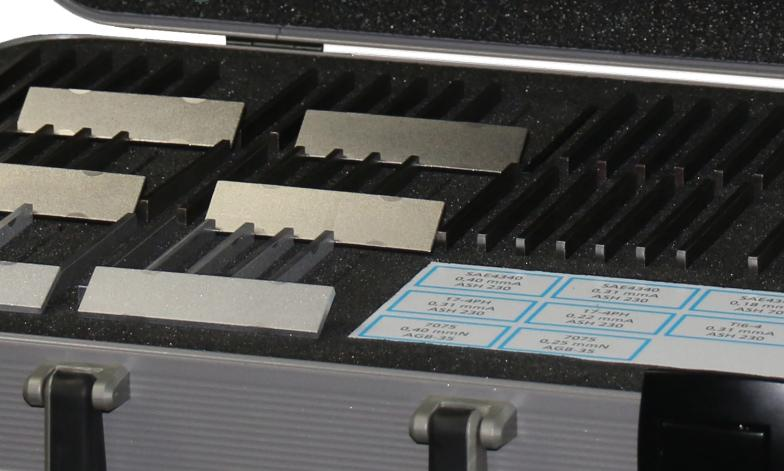
Use of specific comparison samples for coverage development Process-specific radiated reference samples for a simplified assessment of coverage rates in process development, verification and training
